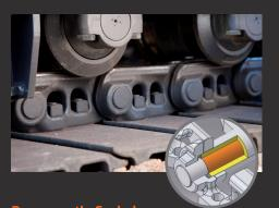
Pin links on tracked DEVELON material handlers are permanently sealed. They never need greasing. That means you reduce your operating costs and increase your uptime. (DX225MH-5, DX300MH-5)
