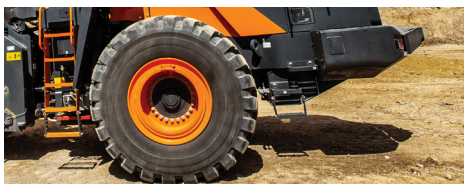
Low sidewall tire - Less sidewall deflection - Improved traction
