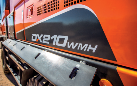
Machine Guarding Strategic guarding on the DEVELON material handler protects components from harsh material and debris, minimizing downtime.
