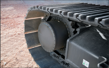
Recessed Drive Motors The drive motors are protected by a heavy-duty cover to protect mobility in severe conditions. On the outside of the tracks, the drive motors are recessed, offering further protection against potential damage while maximizing uptime. (DX300MH-5, DX225MH-5)
