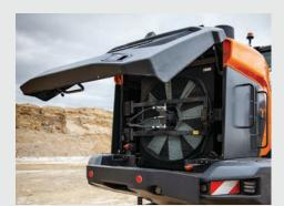
A new radiator with wider fin spacing on some models quickly clears dirt, dust and other large debris to reduce clogging while keeping the cooling system performing consistently – to minimize machine downtime in scrap, forestry and agriculture applications.
