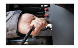
**Centralized lubrication points** make daily greasing more likely to get done. Remote grease points make it easier to lubricate hard-to-reach pins on the lift arm and articulation system.
