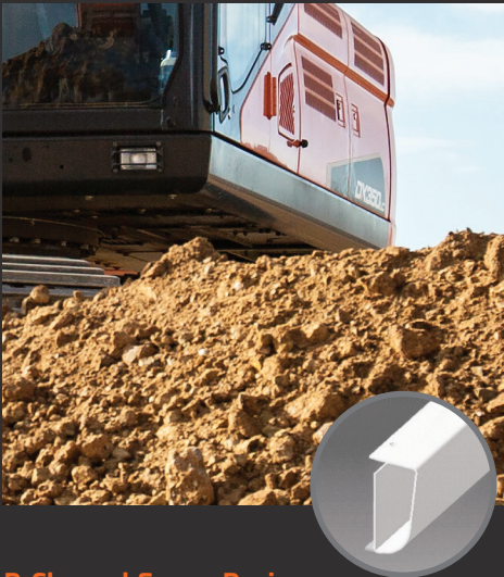
D-Channel Frame Design This innovative upper-structure frame design adds strength to withstand more side shock and protect vital machine components.
