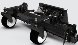
Power Rake Highly effective for grading and leveling uneven terrain like lawns, driveways and construction sites.
